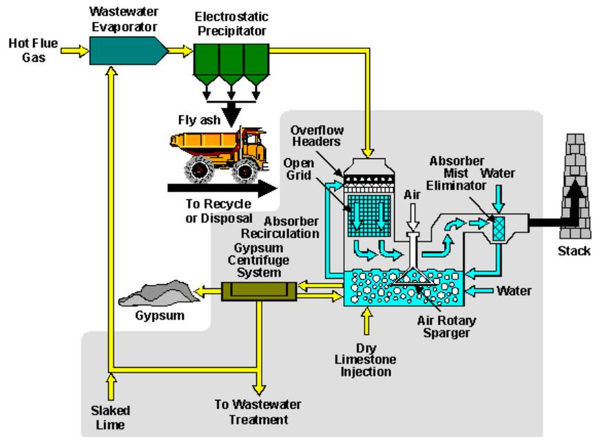
Control systems for primary PM (electrostatic precipitator) and secondary PM precursors (sulfur dioxide scrubber) at coal-fired power plants (Courtesy of US DOE Office of Fossil Energy)
