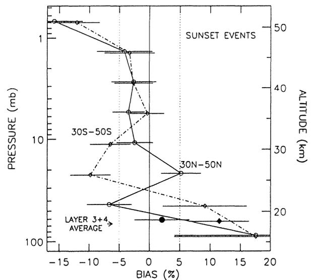
**Figure 1-11.** Ozone profile bias of SBUV relative to SAGE sunset data in northern midlatitudes (o) and southern midlatitudes (◊) for 1984-1990. The solid symbols are for layers 3+4 combined to represent the low SBUV resolution in the lower stratosphere. Standard deviations of the appropriate daily values used in calculating the average biases are also plotted. (McPeters *et al.*, 1994.)
