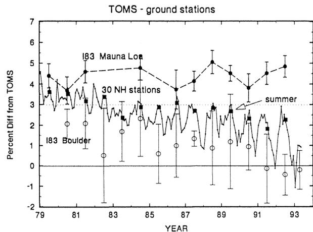
**Figure 1-3.** Percent difference between TOMS and World Standard Dobson #83, at both Mauna Loa (solid circles) and at Boulder (empty circles); monthly average differences for an average of 30 Northern Hemisphere Dobson stations; and summer only (JJA) differences for the same stations (squares). The uncertainties shown are 95% confidence limits for the mean value.
