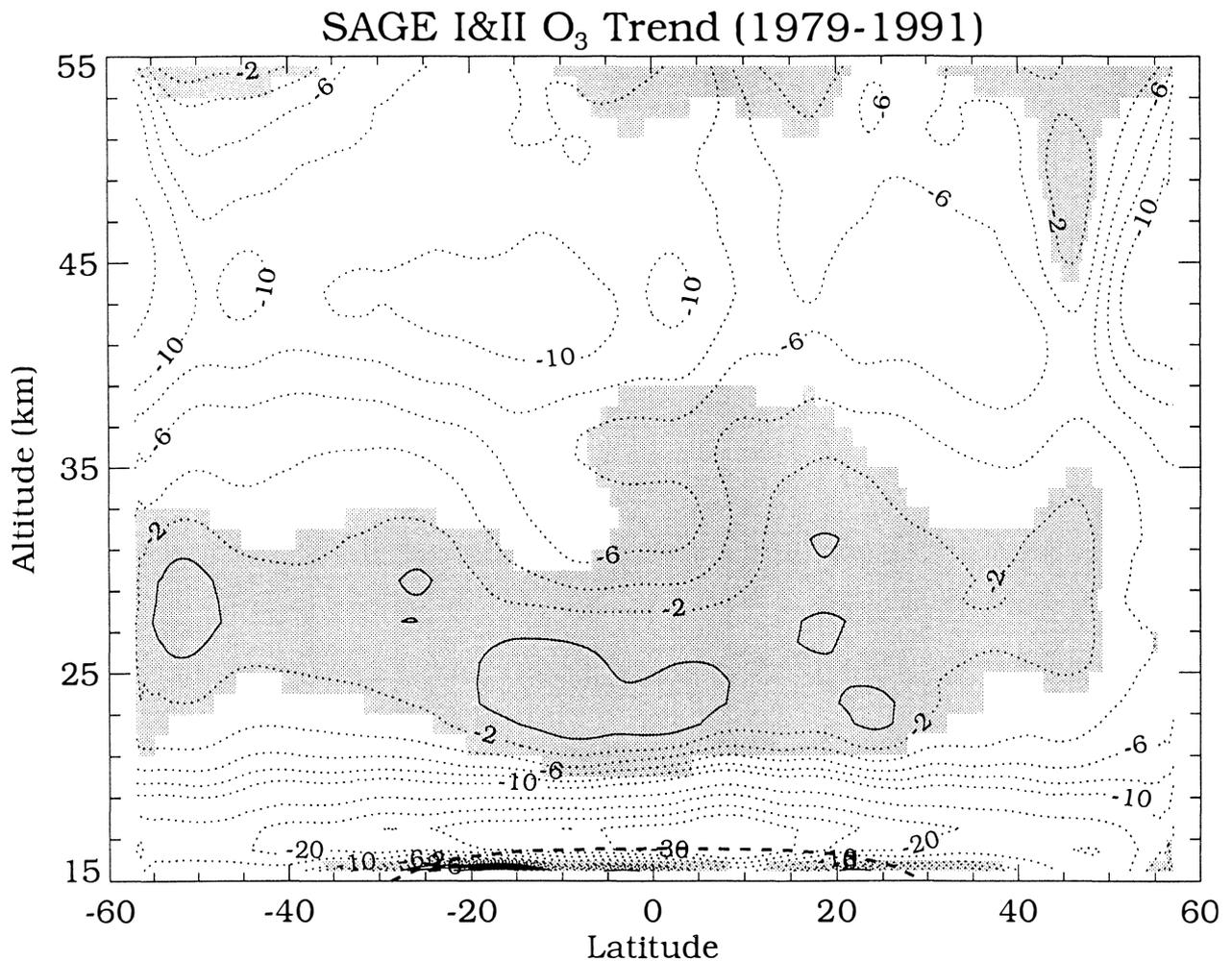
**Figure 1-13.** (b) Trends calculated for SAGE I/II for 1979-91. Hatched areas indicate trends calculated to be insignificant at the 95% confidence level. The dashed line indicates the tropopause. The altitudes of the SAGE I measurements have been adjusted by 300 meters.
