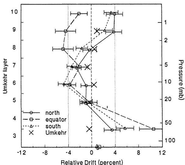
**Figure 1-12.** Linear drift of SBUV relative to SAGE II over the 1984-1990 time interval for layers 5-10 and for layer 3+4 combined, derived from a linear fit applied to difference data. (SBUV-SAGE)/SAGE in percent is plotted. Symbols on X axis give drift of layer 3-10 integrated ozone amounts. For comparison, drift relative to an average of five Umkehr stations (1984-1990) is also shown. The  $1\sigma$  errors from the standard regression analysis are given. (McPeters *et al.*, 1994).
