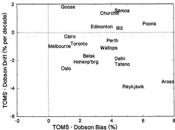
**Figure 1-2.** The average bias relative to TOMS in the first year (usually 1979) and the drift relative to TOMS over 14 years for a sample of 18 Dobson stations. The Dobson station data were taken from the World Ozone Data Center in December 1993. I83 at Mauna Loa and the regular Mauna Loa record are shown separately.
