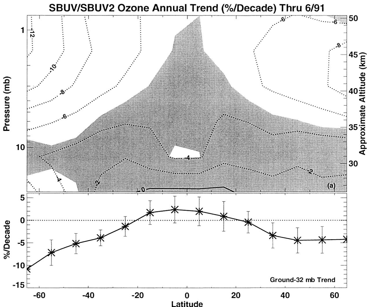
**Figure 1-13.** (a) Trends calculated for the combined SBUV/SBUV2 data set for 1/79 to 6/91. Hatched areas in the upper panel indicate that the trends are not significant (95% confidence limits). The lower panel shows the trends in the partial column between the ground and 32 mbar. Error bars in the lower panel represent 95% confidence levels.
