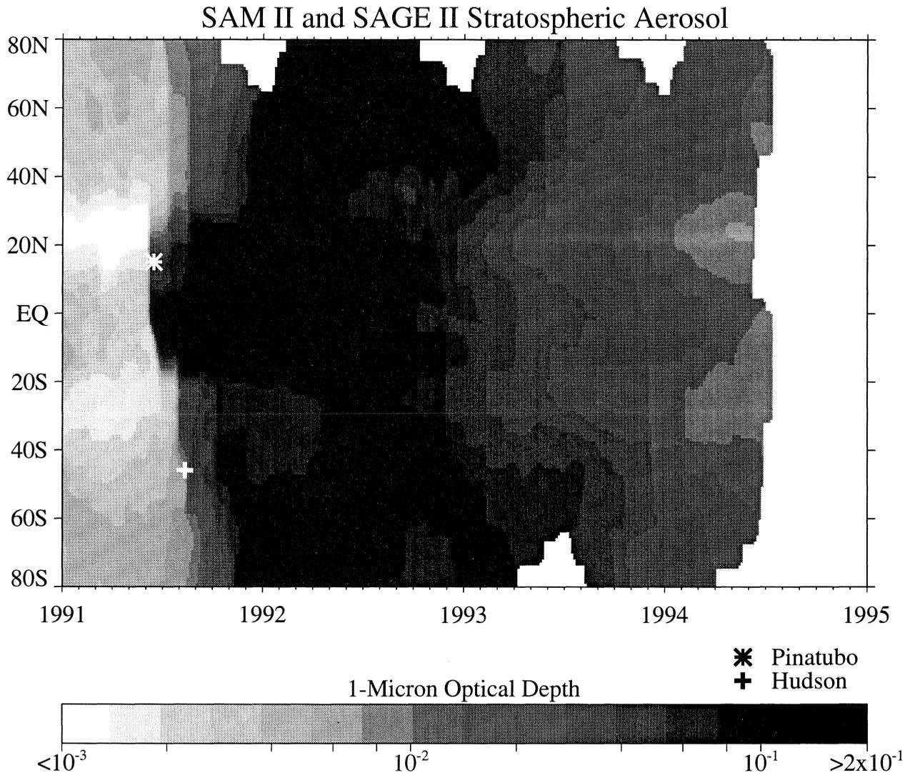
**Figure 1-22.** Aerosol optical depths from 1991-1994 measured by SAM II and SAGE II showing the effects of the Mt. Pinatubo (\*) and Volcán Hudson (+) volcanic eruptions. (Updated by L. Thomason from data shown in Trepte *et al.*, 1993.)
