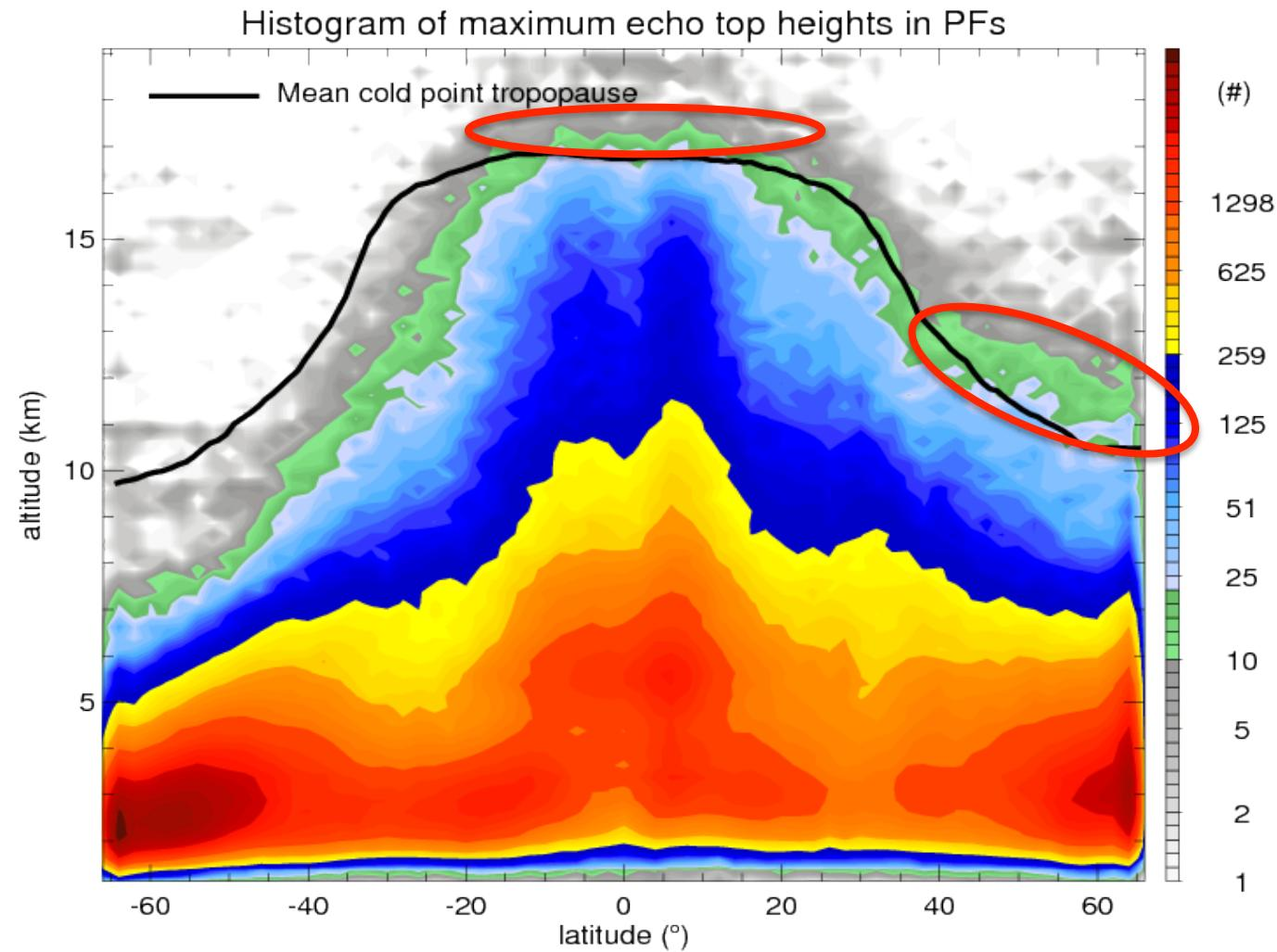
ERA-Interim reanalysis temperature profiles with 6 hourly  $0.75^{\circ} \times 0.75^{\circ}$  resolution are interpolated to PF times and locations, then the cold point tropopause heights are calculated for each PF
