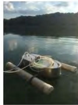
Aluminum floating chamber for measuring diffusive emissions from a reservoir.
