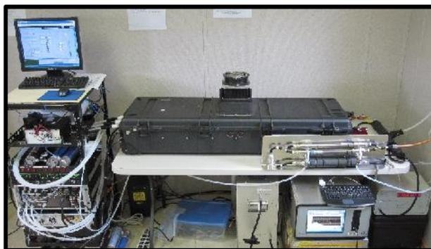
CRDS instrument to measure  $\text{NO}$ ,  $\text{NO}_2$ ,  $\text{NO}_y$ , and  $\text{O}_3$
