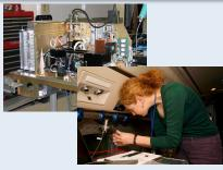
CSD's Single Particle Soot Photometer (SP2) quantifies the refractory black carbon (rBC) mass and mixing-state of individual rBC-containing particles.
