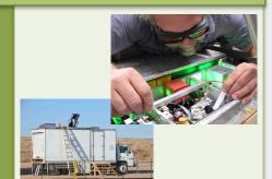
The Tunable Optical Profiler for Aerosol and oZone (TOPAZ) lidar measures ozone and aerosol in the lower troposphere. Aircraft deployments achieve 90-m vertical and 600-m horizontal resolution.
