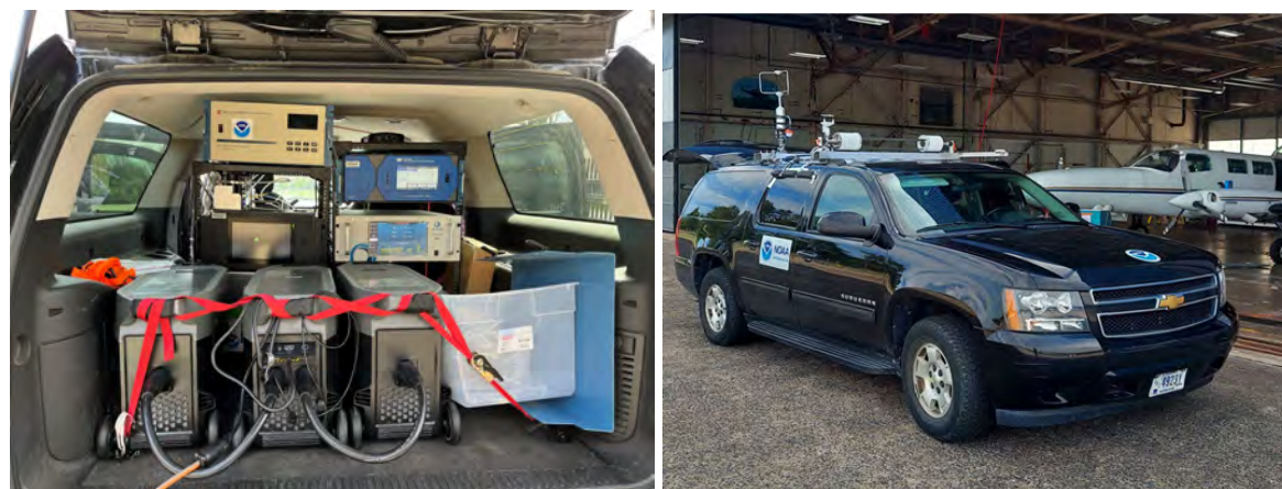
Figure 5. Pictures showing the instrumentation in NOAA's Air Resources Car mobile lab.
