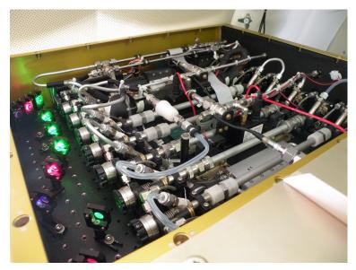
The **AOP** combined instrument package measures the aerosol properties necessary for calculations of radiative forcing and atmospheric heating rates. Further, the measured parameters can be directly compared to those derived from remote sensing measurements from satellite, airborne, and ground-based sensors. Additional measurements, such as the change in aerosol absorption and
