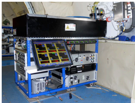
Figure 1. Nitrogen oxide CRDS instrument during CalNex 2010
