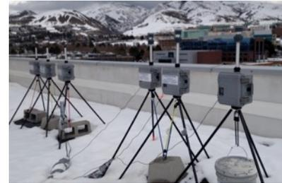
MiniVol PM<sub>2.5</sub> samplers on WBB roof
