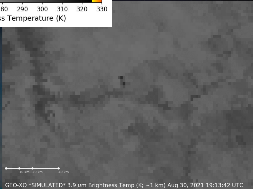
Simulated 3.9 \mu\text{m} 1 km resolution band from GXI for the same times as the ABI loop. It's based on VIIRS passes at 1913 (SNPP), 1959 (N20), and 2050 UTC (SNPP).
