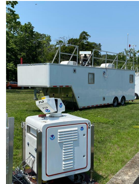
NOAA Doppler lidar and TOPAZ O 3 lidar trailer at YCFS (photo: A. Langford)
