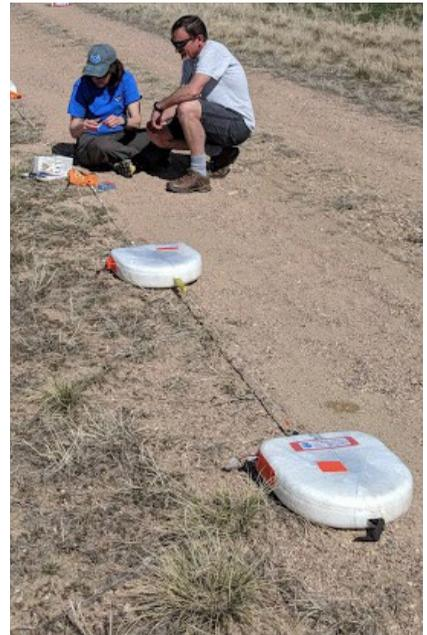
CIRES researchers Sonja Wolter and Jack Higgs prepare the components of an AirCore payload string for air sampling. Photo: Tim Newberger/CIRES
