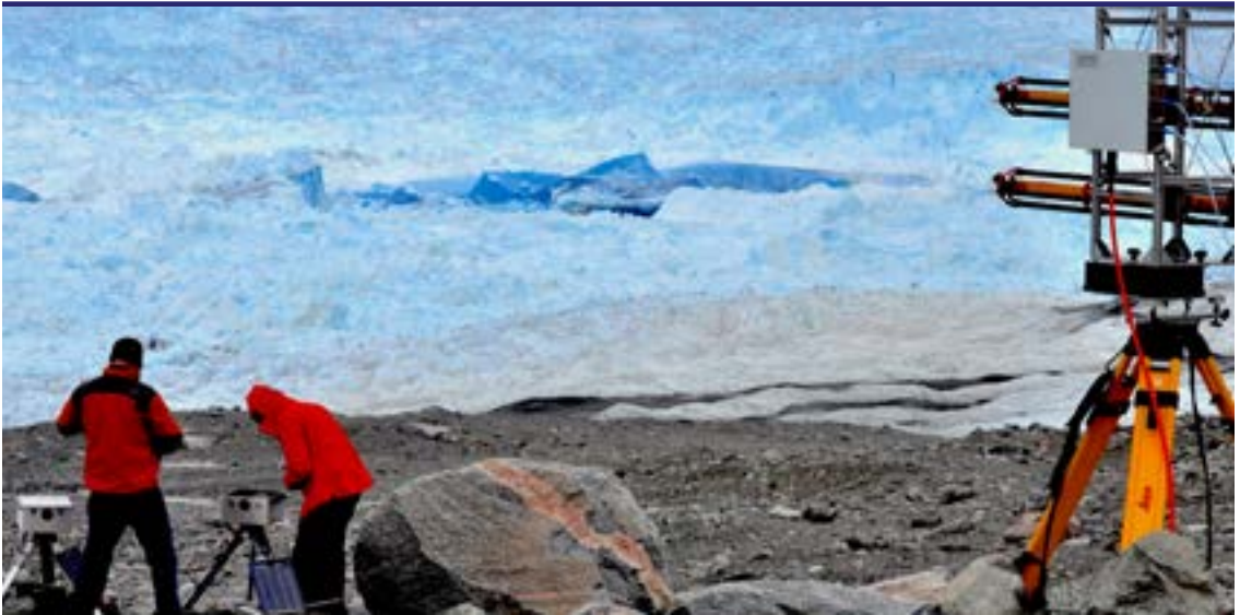
Scientists use time-lapse cameras at the edge of a proglacial fjord in Greenland. At the right is one of ground-based radar interferometers used to record the movement of icebergs. Photo: Ryan Cassotto/CIRES
