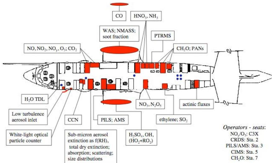
**Figure 15. Proposed 2006 payload for the NOAA WP-3D Orion aircraft.**
