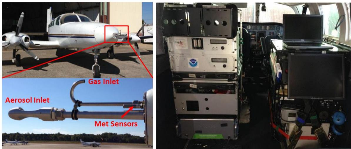
**Figure 3.** The proposed instrumentation on the UMD Cessna for the Baltimore Air Quality and Marcellus Methane Survey in 2025.
