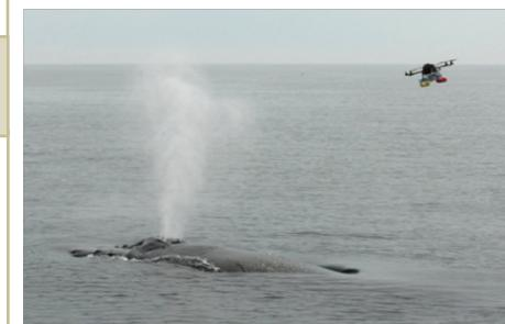
Blow sampling of large whales using APH-22 UAS without disturbance by close boat approach. Source: NOAA
