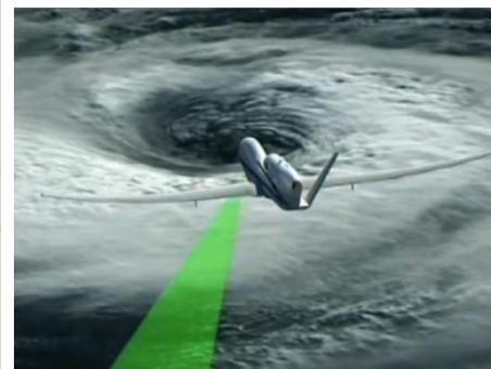
Graphic illustrating the high-altitude, long-endurance Global Hawk UAS platform operating above hurricanes to obtain measurements in and around storms to improve forecast capabilities. Source: NASA
