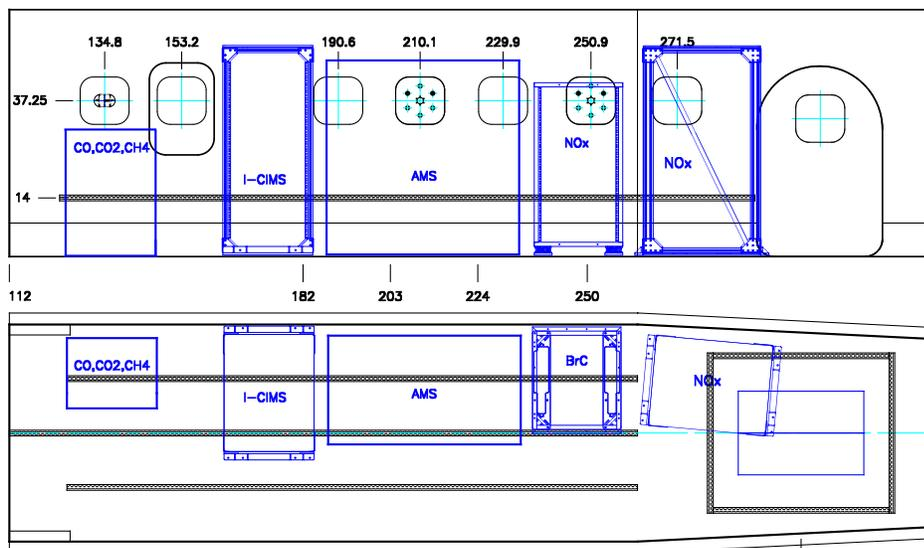
**Figure 5:** The potential payload for the NOAA Twin Otter for FIREX-CHEM: (1) CO, CO<sub>2</sub>, CH<sub>4</sub>, (2) O<sub>2</sub>, NO, NO<sub>2</sub>; (3) I-CIMS; (4) HR-AMS; (5) BrC-PILS.
